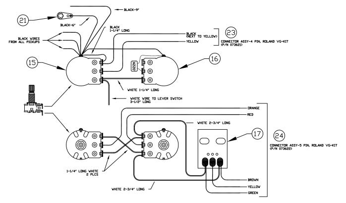
VOLUME POT, TONE POT AND TUNING SWITCH WIRING
